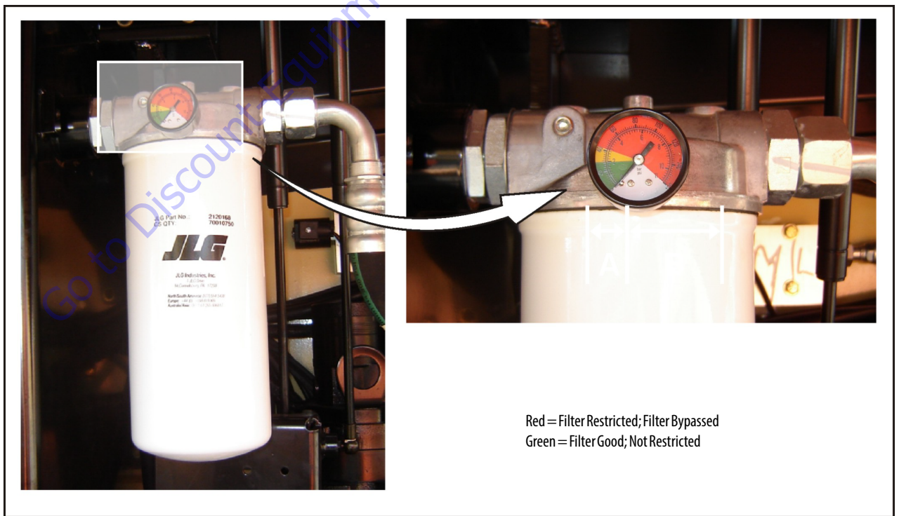
Figure 1-4. Hydraulic Return Filter Condition Indicator - SN 139396 to Present
